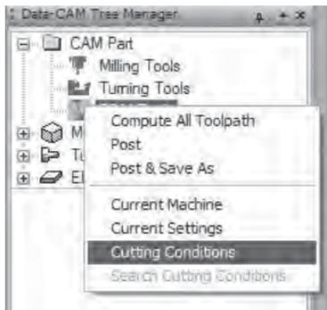
BobCAD-CAM will display the **Edit Cutting Conditions Database** dialog box. At the top of the box will be listed the current **Material**, **Wire Diameter**, and **Stock Thickness**.
