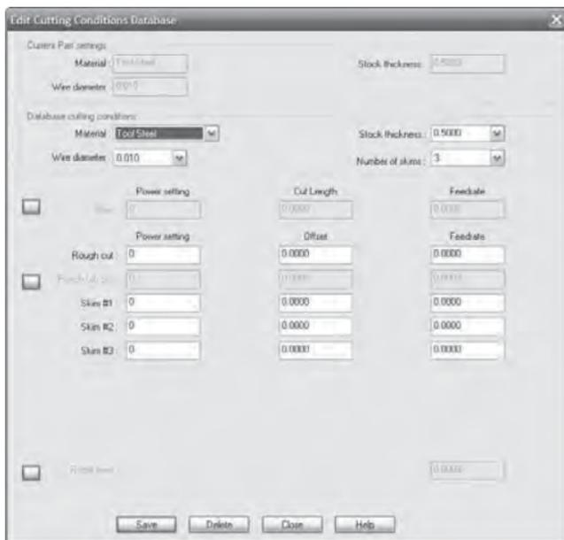
Below that, it is possible to change the **Power Setting**, **Cut Length** and **Feedrate** field for the start of the cut as well as for the rough and skim passes. Choose the **Material** from the list as well as the **Stock Thickness**, **Wire Diameter**, and the **Number of Skins** to edit. If any of the fields below need to be changed, change them and click **Save**. BobCAD-CAM will update the database file for this machine. When finished, click **Close**.
