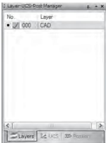
To create a new layer, right-click in the **Layer-UCS-Post Manager** and choose **Add New Layer**. Name the new layer whatever is necessary. BobCAD-CAM Version 23 keeps layers separated in the background by their numbers, not their names, so it is possible to name 2 layers the same if required.
